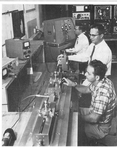
USING A REFLECTOMETER SYSTEM, men of Section 2412-2 measure unknown voltage standing wave ratios of small magnitudes. Microwave reflection coefficients as small as .002 can be measured with this system. From front are Robert L. Kasparek, Ned A. Lindsay, and Paul E. Livingston, who operate instrument.
